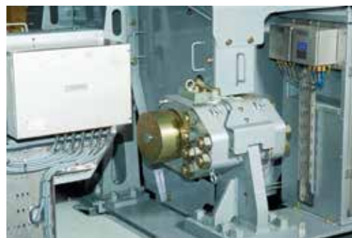
Brake calipers and ATEX-certified hydraulic power units designed by Svendborg Brakes for drawworks have been developed specifically to DNV and ABS standards.
