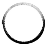
Outermost diaphragm of a coupling that failed due to overly-high misalignment. The rest of the coupling continued to operate for more than 10 million cycles
