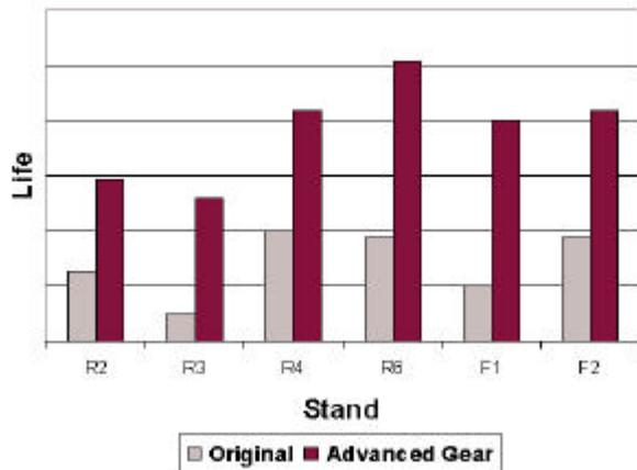
Ameridrives has applied the new design to all mill applications from 3½ inch leveler spindles, 21 inch high speed cold mill spindles to 38 inch hot mill spindles with significant life increases for all applications.
