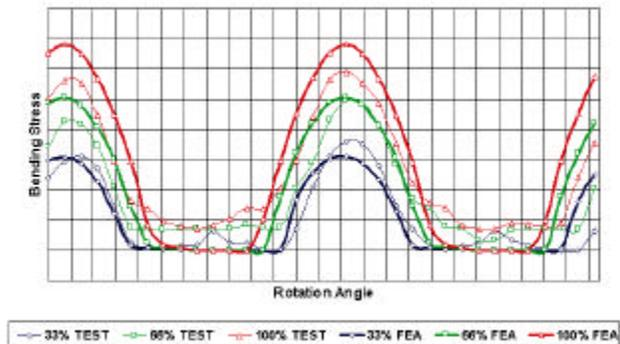
In reviewing Figures 11 and 12, notice that the curves exhibit the same pattern, confirming the percent of teeth in contact method. In addition to this, the actual stress values are also within 15% with the design (FEA) values on the high or conservative side.
