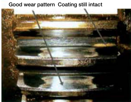
Teflon-coated gear hub.
