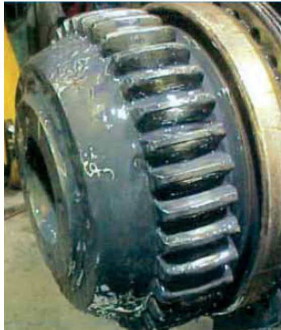
Gear hub dripping with oil.
