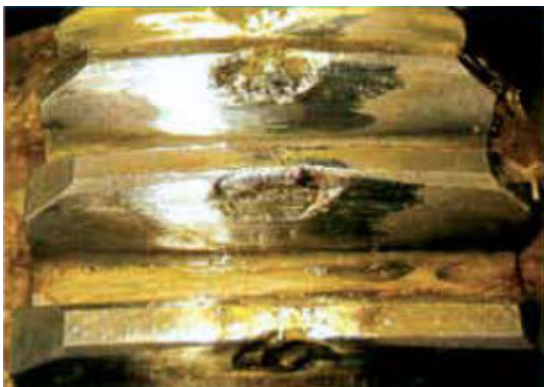
Gear hub after Lyon additive blended with grease.
