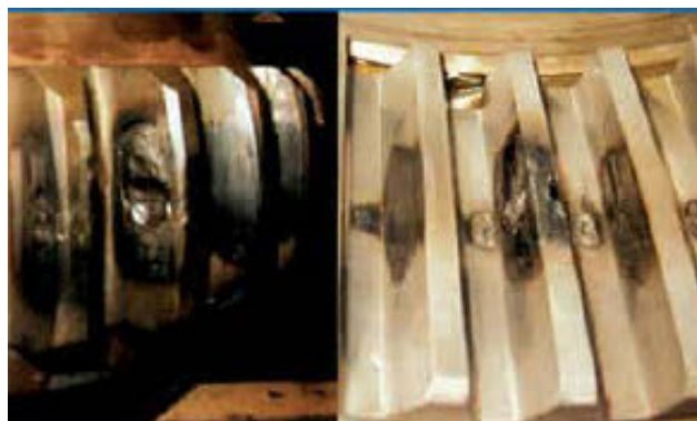
Gear hub and gear ring after synthetic oil trial.
